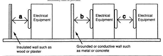
Distances are measured from live parts if they are exposed or from the enclosure front if live parts are enclosed.
